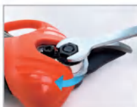
10. Install pins and serrated nuts;
