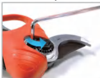
3. Remove the anti loosening gasket screws;
