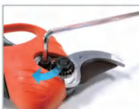
11. Install the anti loosening gasket screws;
