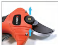
1. Remove the screws from the machine casing;
