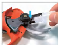
9. Replace the blade and apply lubricating oil;
